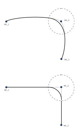
34.1: Joint space (MoveJ) vs. cartesian space (MoveL) movement and blend.
