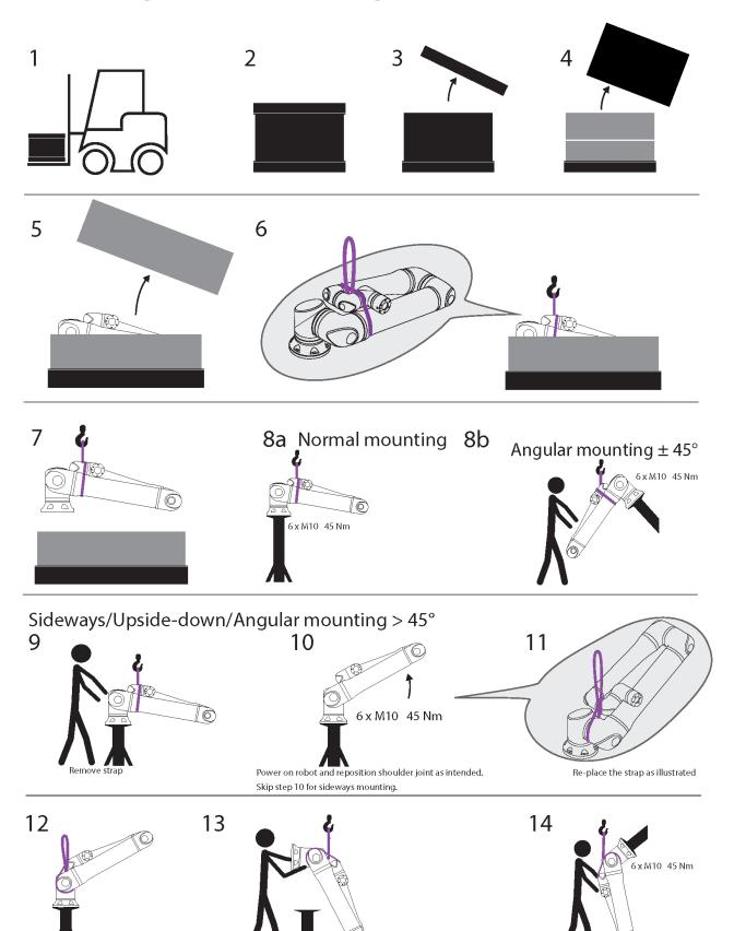
When releasing and lifting the robot, support it to rotate and hang as illustrated
