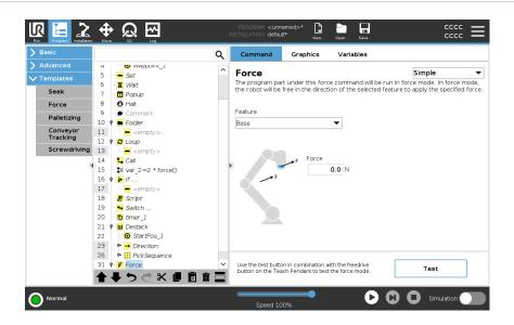
Feature selection The Feature menu is used to select the coordinate system (axes) the robot will use while it is operating in force mode. The features in the menu are those which have been defined in the installation.
