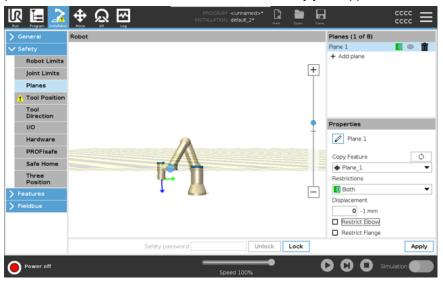
The unrestricted tool flange can cross a safety plane, even when no tool is defined. If no tool is added, a warning on the Tool Position button prompts you to correctly define the tool.
