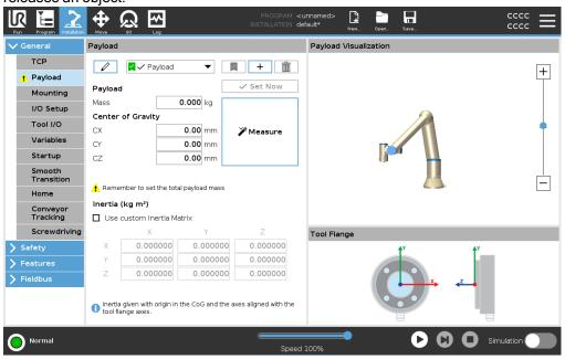
Adding, Renaming, Modfying and Removing Payloads You can start configuring a new Payload with the following actions:
