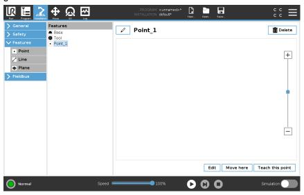
Use Edit to place and move features without moving the robot arm, so the feature can be placed outside of the robot arm's reach.
