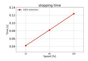
Stopping time in seconds for 66% of 30 kg
