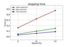
Stopping time in seconds for maximum payload of 30 kg
