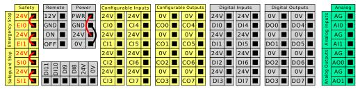
You can use the horizontal Digital Inputs block (DI8-DI11), illustrated below, for quadrature encoding Conveyor Tracking (see Common specifications for all digital I/O on the next page) for these types of input.
