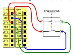
Note: The two input channels for the Three-Position Enabling Device input have a disagreement tolerance of 1 second.
