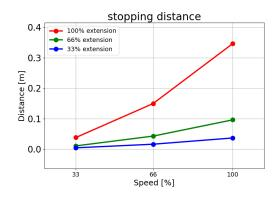
Stopping distance in meters for 66% of 30 kg
