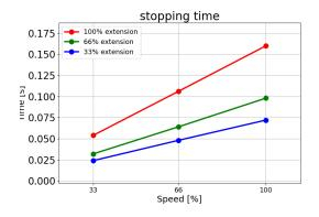
Stopping time in seconds for 66% of 30 kg
