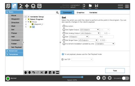
**Set digital output** The digital output should be planned as a start/stop or on/off action.
