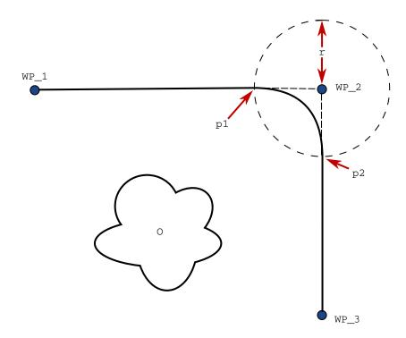
33.2: Blend over  $(WP_2)$  with radius (r), initial blend position at p1 and final blend position at p2. (0) is an obstacle.
