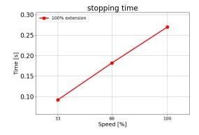
Stopping time in seconds for maximum payload of 30 kg
