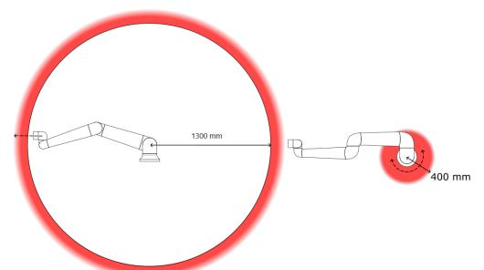
3.1: Due to the physical properties of the robot arm, certain workspace areas require attention regarding pinching hazards. One area (left) is defined for radial motions when the wrist 1 joint is at least 450 mm from the base of the robot. The other area (right) is within 200 mm of the base of the robot, when moving tangentially.
