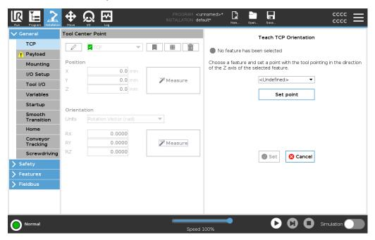
Though three positions are sufficient to determine the TCP, a fourth position can be used to further verify the calculation is correct. The quality of each saved point, with respect to the calculated TCP, is indicated using a green, yellow, or red LED on the corresponding button.
