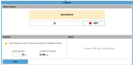
3. Move robot as in Freedrive mode. Joint brakes are released where needed once the Freedrive button is activated.
