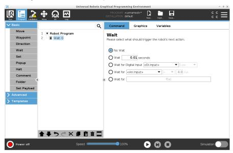
The No Wait command can be used a temporary placeholder be used, when you are programming your robot program.
